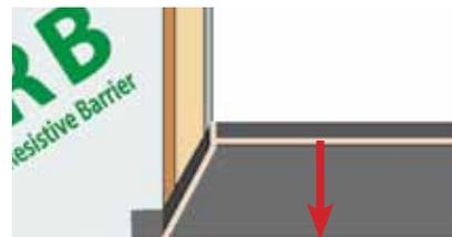
Just before installing the door, apply one 3/8" continuous bead of sealant, from end to end, along the back vertical lip of the sill pan.
