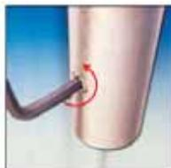
Loosen set screws B & C of bottom knuckle with 2.5 mm Allen key.
