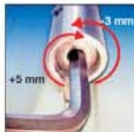
Make adjustment up & down with 5 mm Allen key. CW=Up CCW=Down
