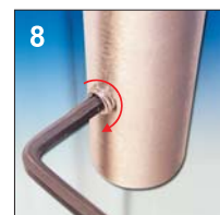
8 Tighten both set screws with 2,5 mm Allen key.
