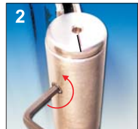
2 Loosen the set screw with 2,5 mm Allen key.
