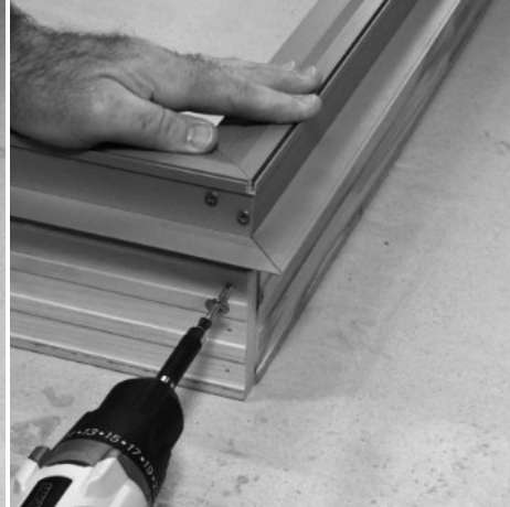
Tighten snug - Do not over-tighten
