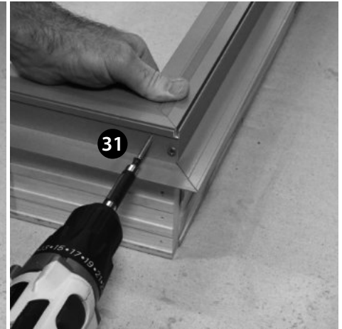
Second Fastener (31) at other hole
