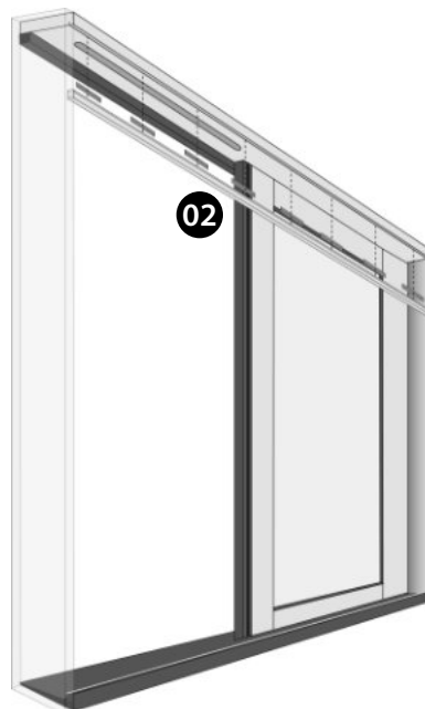
Interior Head Stop Location in Head Jamb
