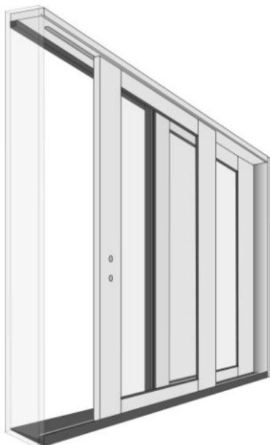
Stand The Panel Upright In The Frame
