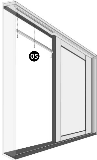
Wind Load Bar Location in Head Jamb
