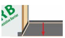
Just before installing the door, apply one 3/8" continuous bead of sealant, from end to end, along the back vertical lip of the sill pan.
