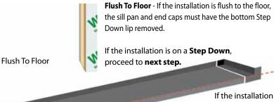
is **Flush To The Floor**, trim off the overhanging Step Down lip from the sill pan and the left and right end caps.
