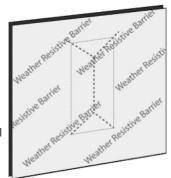
b) Fold weather resistive barrier into the sides and sill. Fold side and bottom flaps into the opening and staple in place.
