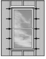
ATTENTION! Do not over-shim or under shim. Do not shim above the window. Proper shimming is required for correct operation and optimum performance of the window.
