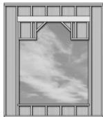
a) Verify rough opening size. The rough opening should provide approximately 1/4" clearance between the sides and top of the product and the framing.
