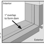
f) Apply sill dam. Cut a second piece of flashing tape the same length as the one used in Step 2d. This will function as a dam against water flowing to the inside if it somehow reaches the sill. Apply to the sill overlapping the first piece 1", with the remainder of the flashing tape extending to the inside. Trim excess at the interior edge.
