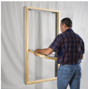
13. Lift up one edge of the sash until the bottom of the sash is clear from the Sash Pivot Shoe in the Side Jamb Track.
